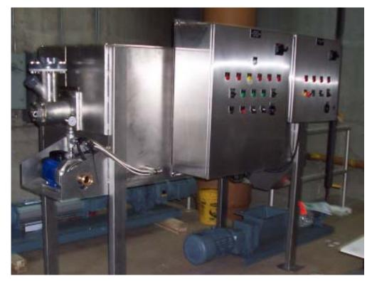
The dewatering results are much higher than with conventional systems. The filter cloth is kept clean by making use of washing water at high pressure from outside. Since it is not under tensile stress, the filter cloth has a long life. To minimize installation time and costs, the Rotary Drum Thickener is supplied as a complete assembled and tested unit.
