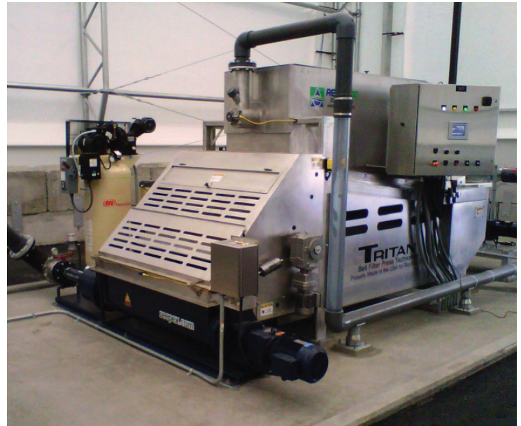
The Tritan discharges a biosolids cake with a solid concentration of 15-20%.
