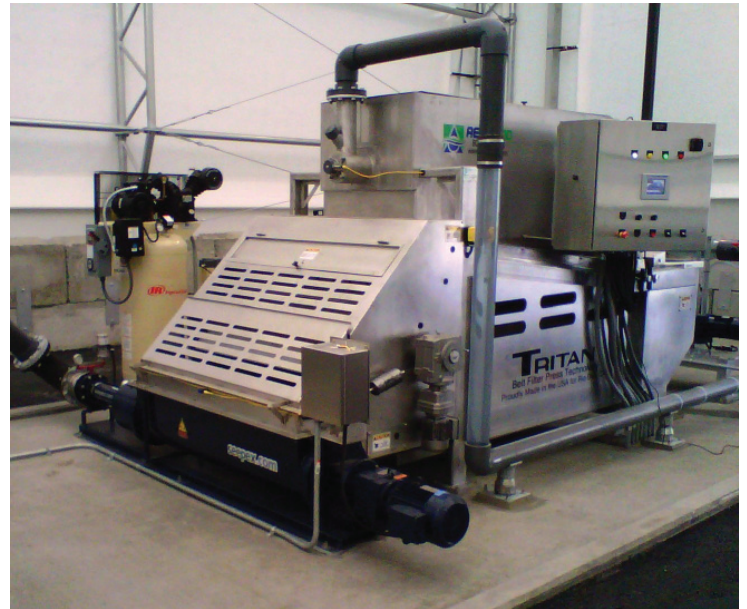
The Tritan discharges a biosolids cake with a solid concentration of 12-16%.
