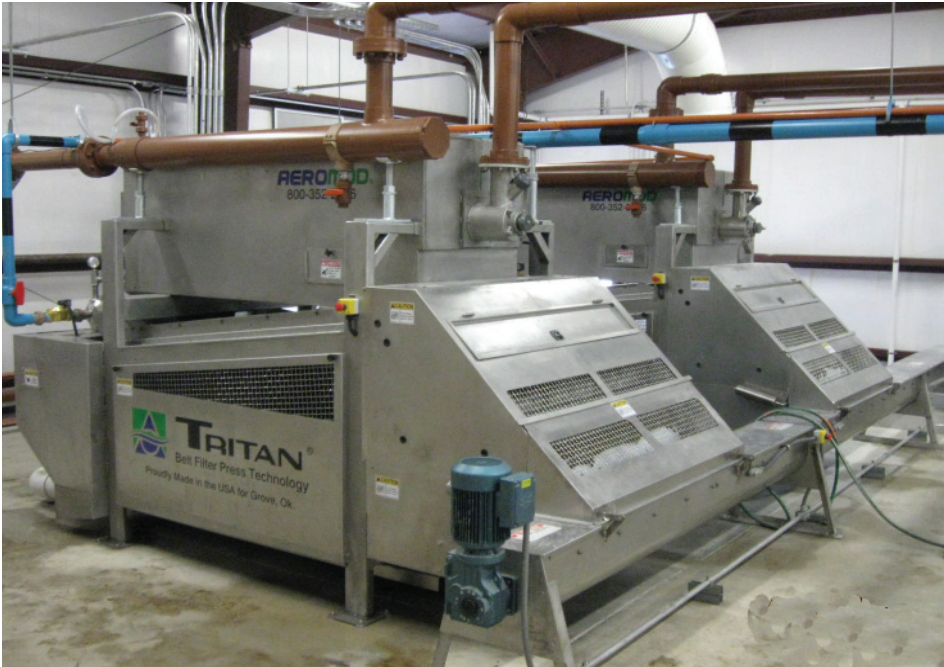
The Tritan™ dewatering belt press provides three belt performance with single belt tracking.
